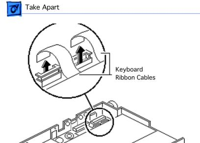
**Caution:** The keyboard ribbon cables are fragile and should be handled with care.
