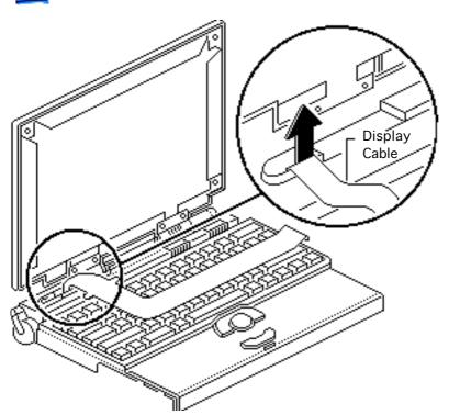
Remove the display cable from the case.
