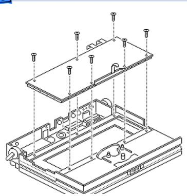
2 Using a T-8 torx driver, remove the seven mounting screws and lift the keyboard from the top case.
