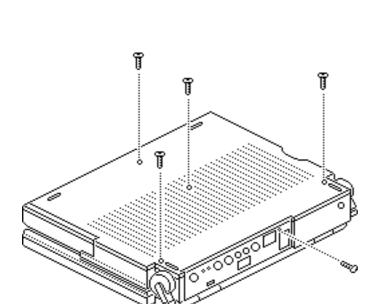
**Note:** Use a T-8 torx driver to remove the small screw from the rear connector panel and a T-10 torx driver to remove the other case screws.
