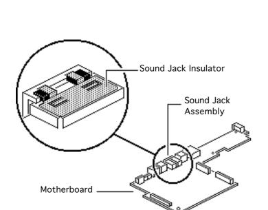
Replacement Note: If you are replacing a defective daughterboard in a PowerBook 160/180 within the serial number range FC233xxxxx through FC241xxxxxx, you must also replace the sound jack insulator on the motherboard.
