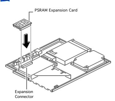
1 Connect the PSRAM expansion card to the expansion connector on the daughterboard.
