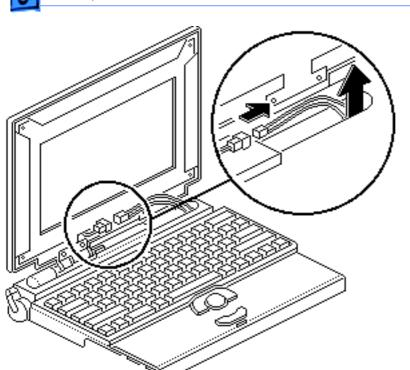
Replacement Note: To avoid pinching the inverter cable, route the cable behind the top-right corner of the hinge on the right clutch.
