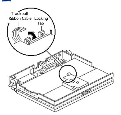
**Caution:** The trackball ribbon cable is fragile and should be handled with care.
