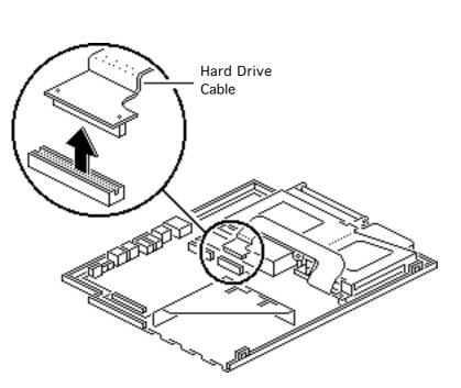
**Caution:** The hard drive cable is fragile and should be handled with care.
