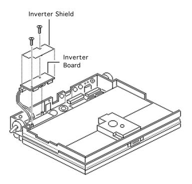
Replacement Note: If you are replacing the inverter board, order both the inverter board and the inverter shield. Install the new shield on the board before replacing it. Do not reuse the original inverter shield.
