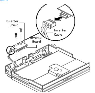
Remove the two mounting screws.
