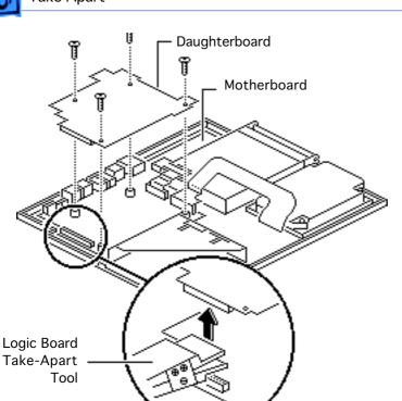
Using a T-8 torx driver, remove the four daughterboard mounting screws.
