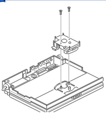
2 Using a T-8 torx driver, remove the two mounting screws and lift the trackball assembly from the top case.
