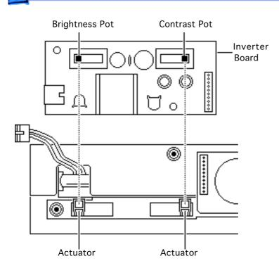
Replacement Note: Be sure to align the brightness and contrast pots on the inverter board with the plastic actuators on the top case. It is easiest to align the pots and actuators if you set both to their extreme outer positions.
