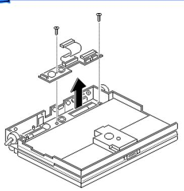
3 Using a T-8 torx driver, remove the two mounting screws and lift the interconnect board from the top case.
