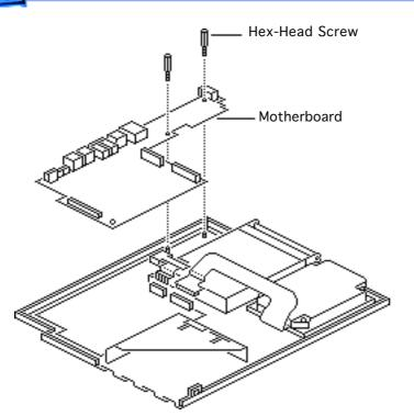
3 Remove the two hexhead screws and lift the motherboard from the bottom case.
