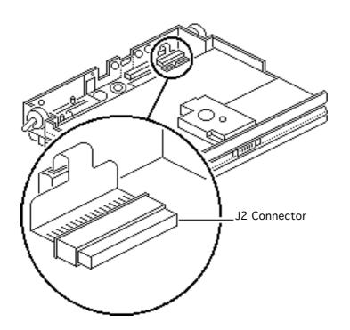
Note: The display cable will not come entirely out of the connector until you remove the interconnect board from the top case.
