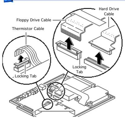
**Caution:** The hard drive, floppy drive, and thermistor cables are fragile and should be handled with care.
